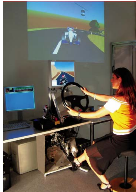
Figure 13 MechatronicCarLab with force-reflecting steering input devices (steering wheel, joystick) and force-reflecting accelerator pedal, real-time vehicle dynamics simulation and visualization
