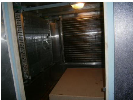
Figure 2 - The interior of the test chamber – preview of evaporator
