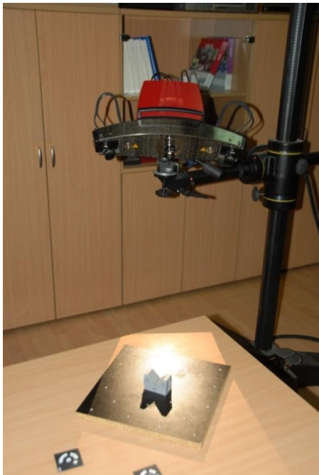
Figure 1 - Digitizing of models with high-end industrial 3D scanner ATOS
