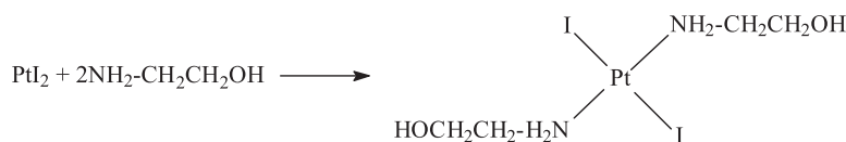
Scheme 1. Synthesis of trans -diiodidobis(2-hydroxyethylamine)platinum(II).
