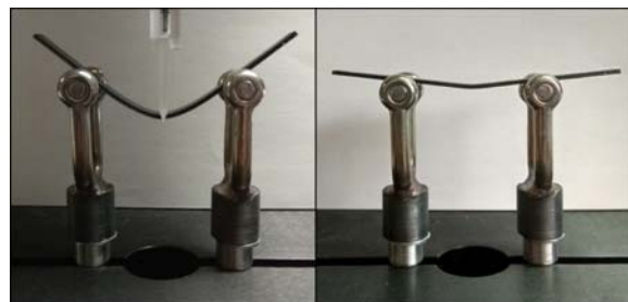
Fig.5. Maximum bent sample (left), sample after relaxation (right)
