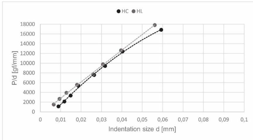
Figure 6. Correlation between P/d and d in accordance to PSR model: a) non-heat treated; b) heat treated;
