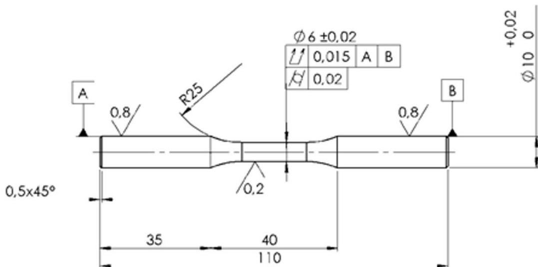
Figure 1. Specimen dimensions in accordance to ISO 1143 standard
