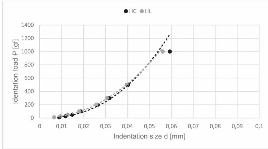
Figure 5. Correlation between P and d in accordance to Meyer's model: a) non-heat treated; b) heat treated
