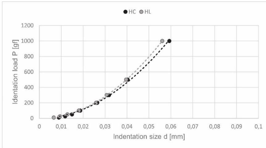
Figure 7. Correlation between P and d in accordance to modified PSR model: a) non-heat treated; b) heat treated
