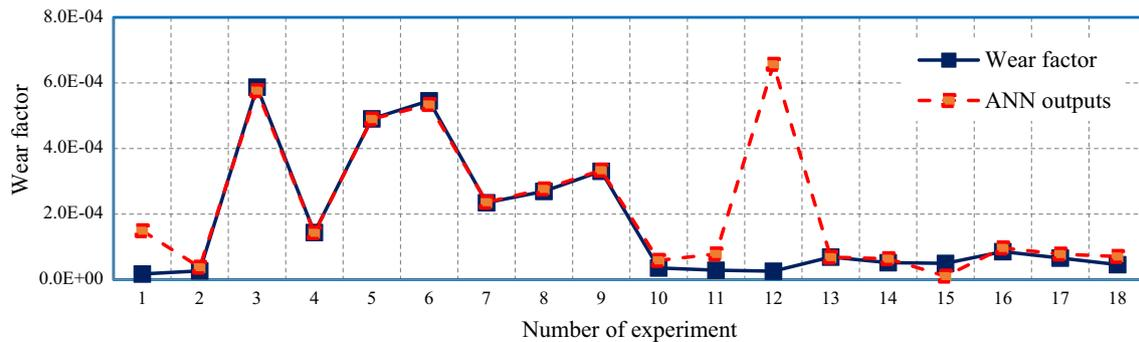
**Fig. 11** Comparison of experimental results with the results of ANN-based model
