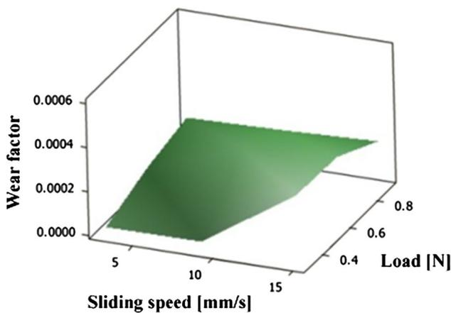
**Fig. 9** Surface plot for showing dependence between wear factor of the load and sliding speed
