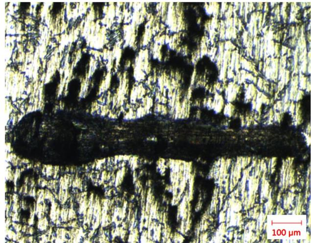
**Fig. 1** Surface micrograph of base material after dry sliding test under ( $F_N = 0.6$  N;  $V = 15$  mm s<sup>-1</sup>)
