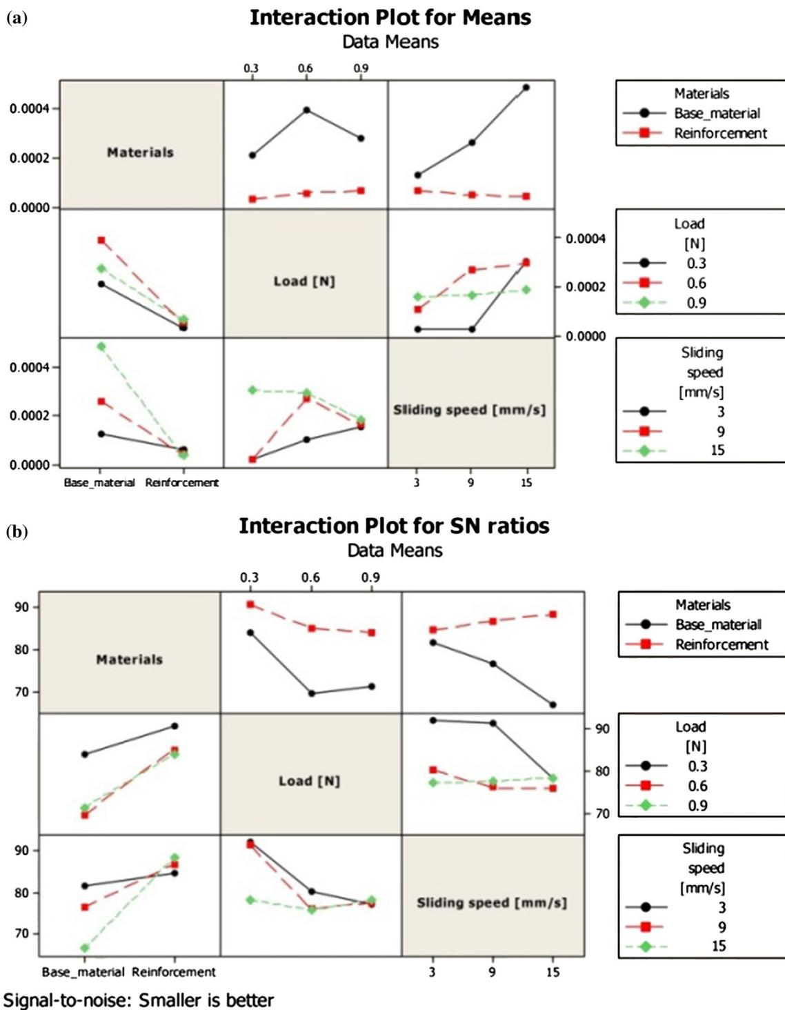
Fig. 7 Interaction plot for: a means—wear factor and b S/N ratio—wear factor
