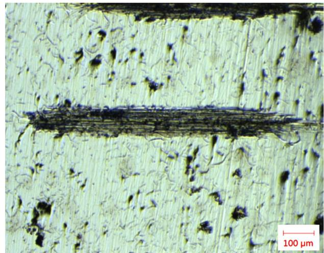
**Fig. 2** Surface micrograph of reinforcement after dry sliding test under ( $F_N = 0.6$  N;  $V = 15$  mm s<sup>-1</sup>)
