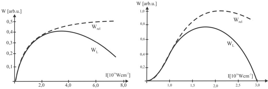
**Fig. 1** Relativistic  $W_{rel}$  (dotted line) and Lorentz  $W_L$  (solid line) transition rates as a function of the laser field intensity,  $I$ , for argon atom  $Ar$ . Intensity varies within the range:  $I = 10^{15} - 8 \times 10^{16} Wcm^{-2}$  **a**  $Z = 1$ , **b**  $Z = 3$
