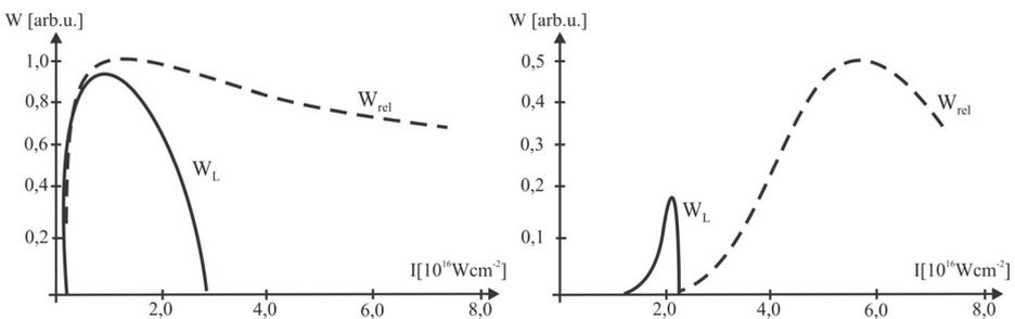
**Fig. 4** Relativistic  $W_{rel}$  (dotted line) and Lorentz  $W_L$  (solid line) transition rates as a function of the laser field intensity,  $I$ , for potassium atom,  $K$ . Intensity varies within the range  $I = 10^{15} - 8 \times 10^{16} \text{ W cm}^{-2}$  **a**  $Z = 2$  **b**  $Z = 3$
