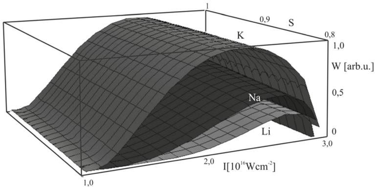
**Fig. 5** 3D graph for  $W_L$  as a function of the field intensity,  $I$  and the stabilization factor  $S$ , for alkali, double ionized,  $Z = 2K, Li, Na$ . Intensity varies within the range  $I = 10^{15} - 8 \times 10^{16} Wcm^{-2}$  and the stabilization factor  $0.8 \leq S \leq 1$
