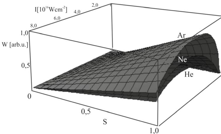
**Fig. 2** 3D graph for  $W_L$  as a function of the field intensity  $I$  and the stabilization factor  $S$  for noble single ionized,  $Z = 1$  argon, neon and helium atoms. Intensity varies within the range  $I = 10^{14} - 8 \times 10^{16} Wcm^{-2}$  and the stabilization factor  $0 \leq S \leq 1$
