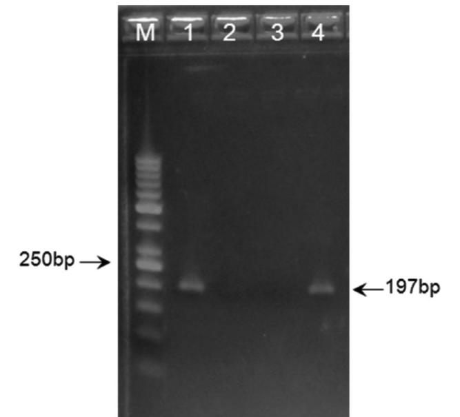
**Fig. 5.** Effects of template DNA concentration on the polymerase chain reaction (PCR) amplification. Lane M: 50 bp DNA ladder; lane 1: 11.3 µg/ml; lane 2: 1.0 µg/ml; lane 3: 1.4 µg/ml; lane 4: 5.7 µg/ml.
