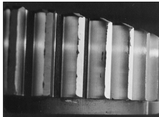
Figure 3. Appearance of the tooth regenerated by hard-facing.
