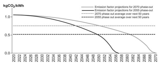
Figure 6. The  $\rm CO_2$  emission factor projections for Serbia for the next 50 years for coal-based electricity phase-out, until 2070 (powerplants lifetime) and until 2055 (early or optimistic)
