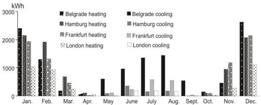
Figure 4. Modelling results of the impact of weather data/location on energy consumption (kWh) of "Smarter Building" building in four hypothetical cases;
