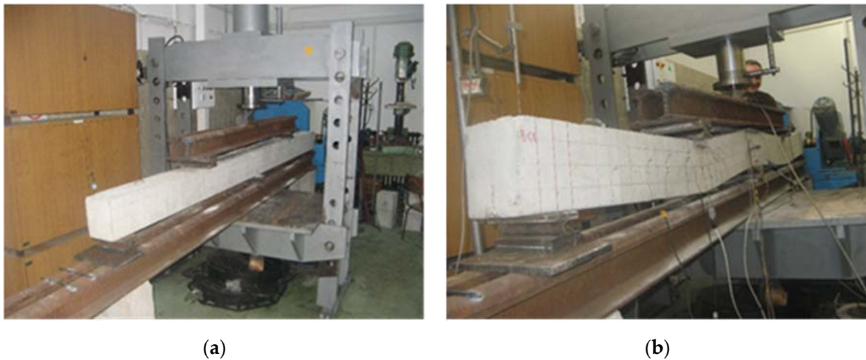
Figure 9. Disposition of the control beam: (a) Before loading; (b) Under loading.
