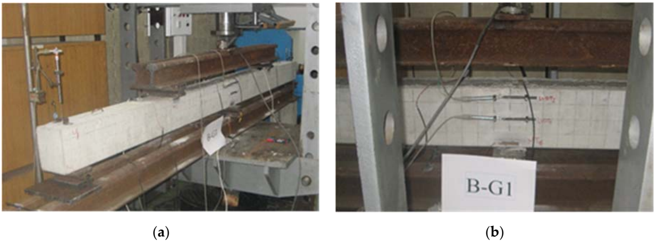
Figure 7. (a) Deflectometer U_1 (LVDT); (b) Dilatometer positions.
