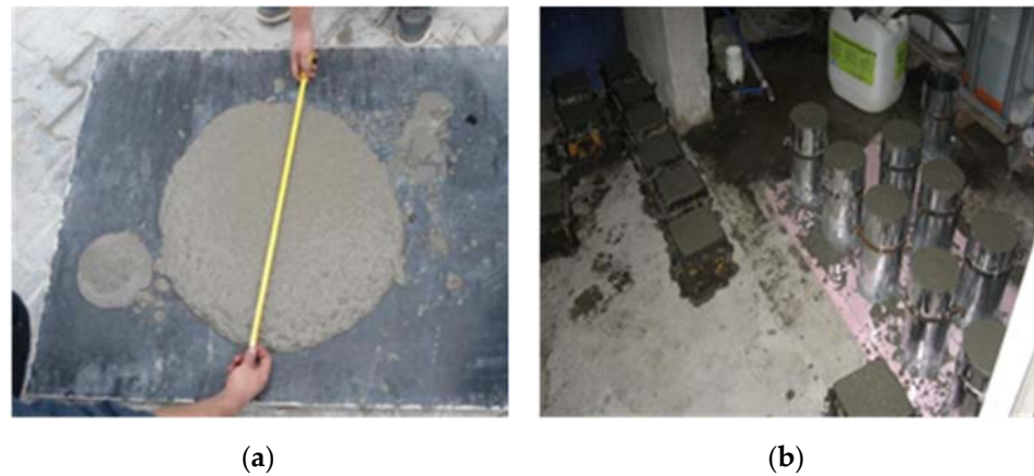
Figure 3. (a) Slump-flow test; (b) Concrete cubes and cylinders.
