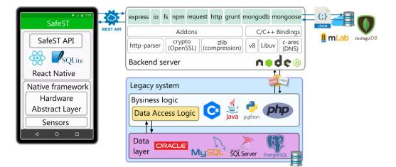
Figure 1. Software architecture of the system.
