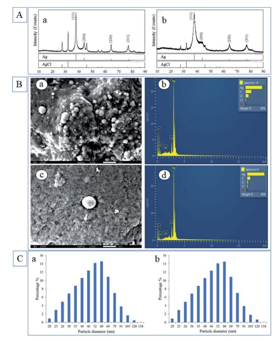
Fig. 3 (A) XRPD pattern of synthesized LSA-AgNPs (a) and LSR-AgNPs (b), (B) SEM image of biosynthesized LSA-AgNPs (a), LSR-AgNPs (c), and their corresponding EDX spectra (b and d), (C) particle size distributions of LSA-AgNPs (a) and LSR-AgNPs (b).
