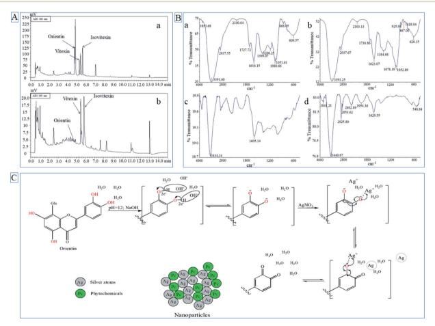
Fig. 2 (A) HPLC-PDA chromatograms of *L. salicaria* aerial part (a) and root (b) aqueous extracts, (B) FT-IR spectra of *L. salicaria* aerial part (a) and root extracts (b) and synthesized nanoparticles LSA-AgNPs (c) and LSR-AgNPs (d), (C) proposed mechanism of orientin Ag(i) reduction during nanoparticle synthesis.
