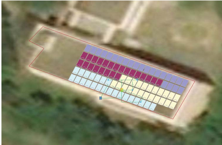
Sl. 2. Raspored fotonaponskih panela na spratnom delu posmatranog objekta Fig. 2. Arrangement of photovoltaic panels on the first floor of the observed building
