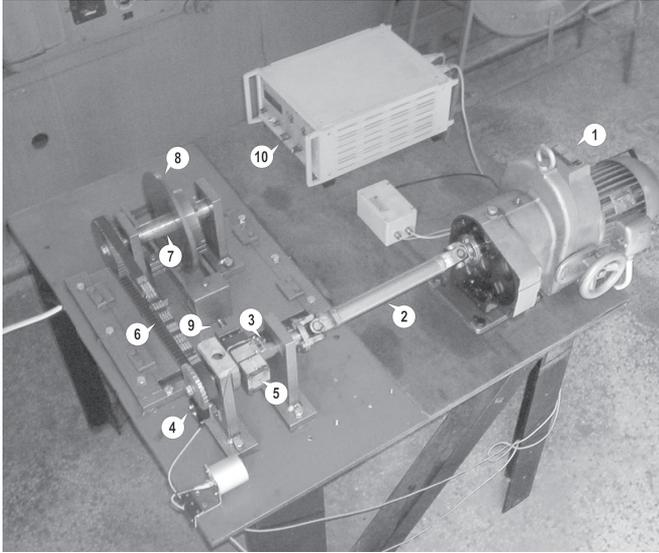
**Fig. 1.** Test bench for testing of timing belt
