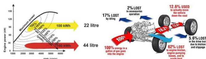
Fig. 2 Diagram of the relative fuel consumption of a typical internal combustion engine and the paths of energy through a typical gas-powered vehicle in city driving [9].
