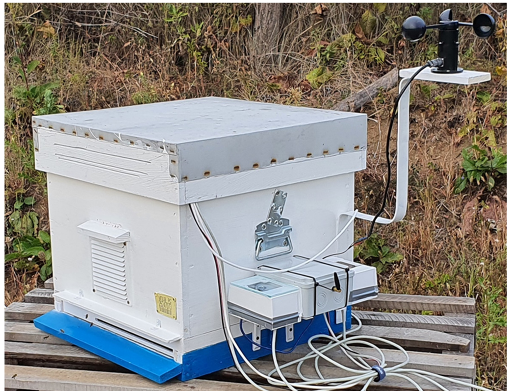
Figure 2. Experimental hive setup with sensor electronics.
