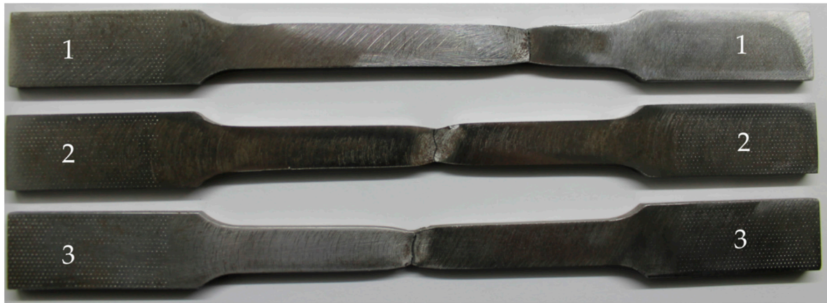
Figure 9. S355J2+N steel specimens after the experimental uniaxial tests.
