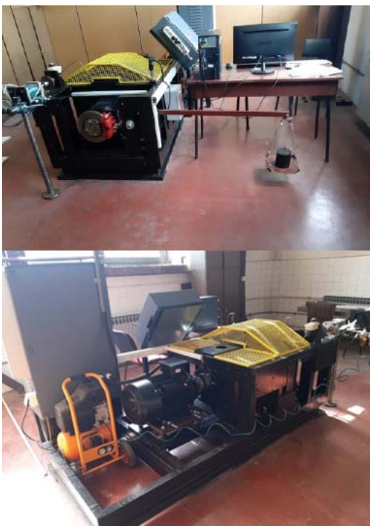
Fig. 20. Inertial brake dynamometer at the Faculty of Engineering [27]
