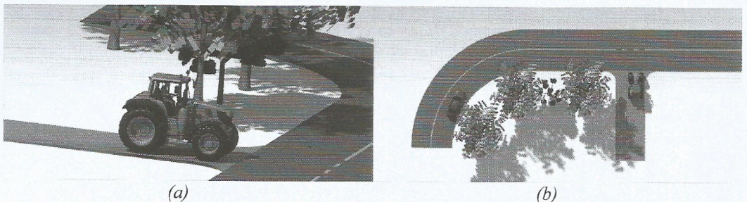
Fig. 6 The representation of the situation when tractor comes out on the main road (a) at right side of the driver (b) from top
