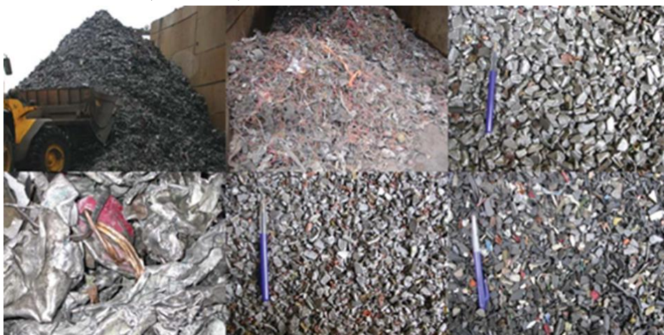
Figure 5: Products of recycling old vehicles in Shredder plant
