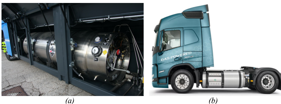
Sl. 2 Ugradnja rezervoara za TPG (a) na međugradskom autobusu i (b) na šasiji tegljača Fig. 2 Installation of LPG tank (a) on an intercity bus and (b) on a tractor chassis
