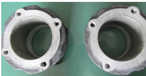
Fig. 4. Photography of cylinders coated inside by Rotaplasma® process before experiments.
