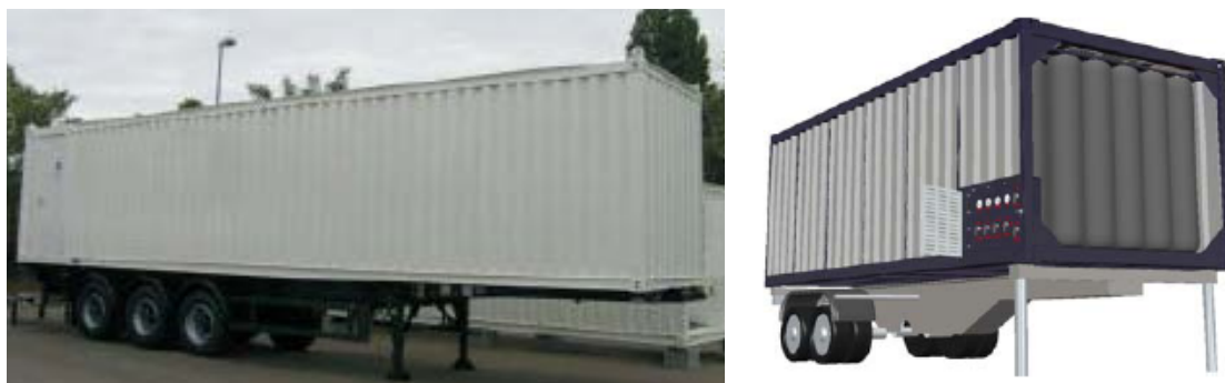
Figure 6. The 250 bar Modules with Cylinders DTK for CNG Bulk Transport [2]
