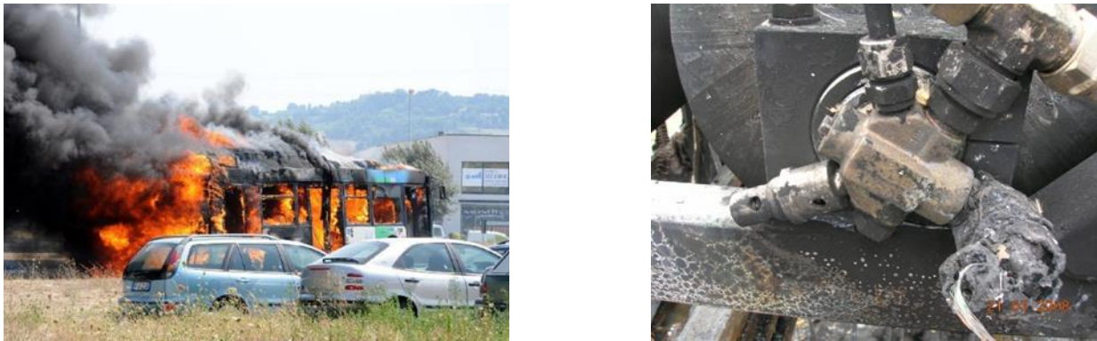
Figure 4 CNG bus under fire (left) and PRD which were successfully activated in a fire (right)
