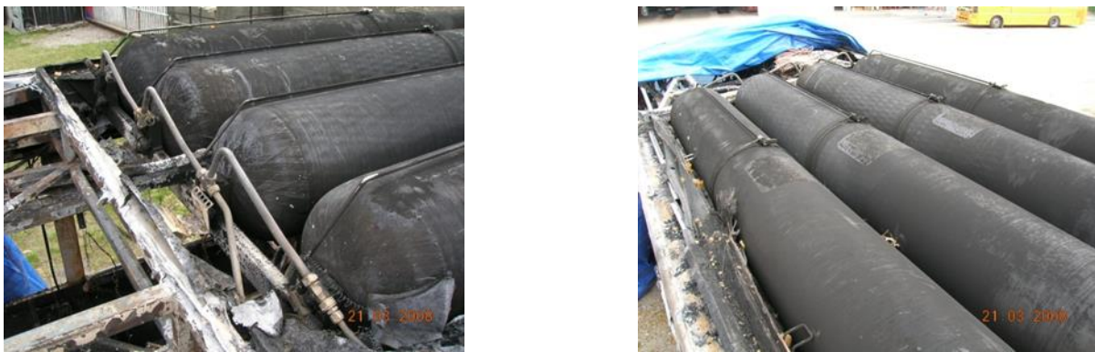
Figure 6 These CNG cylinders were prevented from failing by PRDs which were successfully activated in a fire
