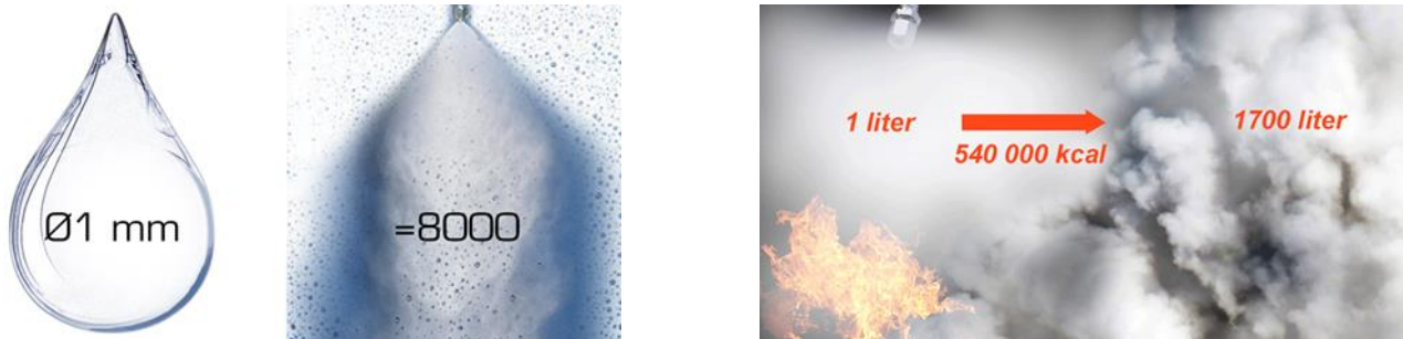
Figure 9 Normal sized water drop vs. water mist and extinguishing fluid water mist effects
