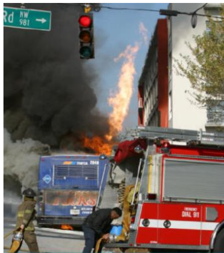
Figure 3 Long and intense jet flame in a CNG bus fire (Jet flame direction is good, but still perilously close to inhabited building)
