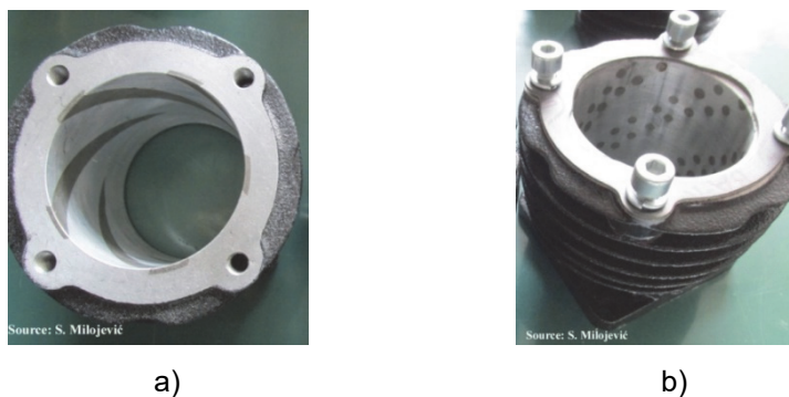
Fig. 2 Photography of patented aluminum cylinder with tribological pads (a-continual and b-nodular discrete pads)
