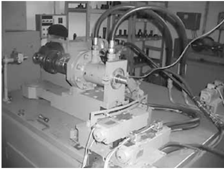
Fig. 3. Laboratory tables for dynamic testing the bearings
