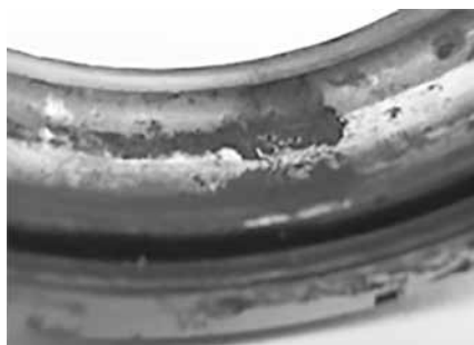
Fig. 10. Fretting corrosion on the outside of the track ball bearing
