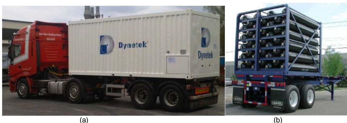
Fig. 5. The 250 bar modules (a) ISO 20 ft. Container (b) 10 ft. cube for bulk transport.
