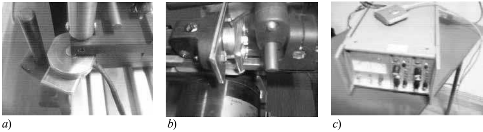
Fig. 3. Measuring force using force sensors: a) input force sensor; b) output force sensor; c) signal amplifier and system for data acquisition
