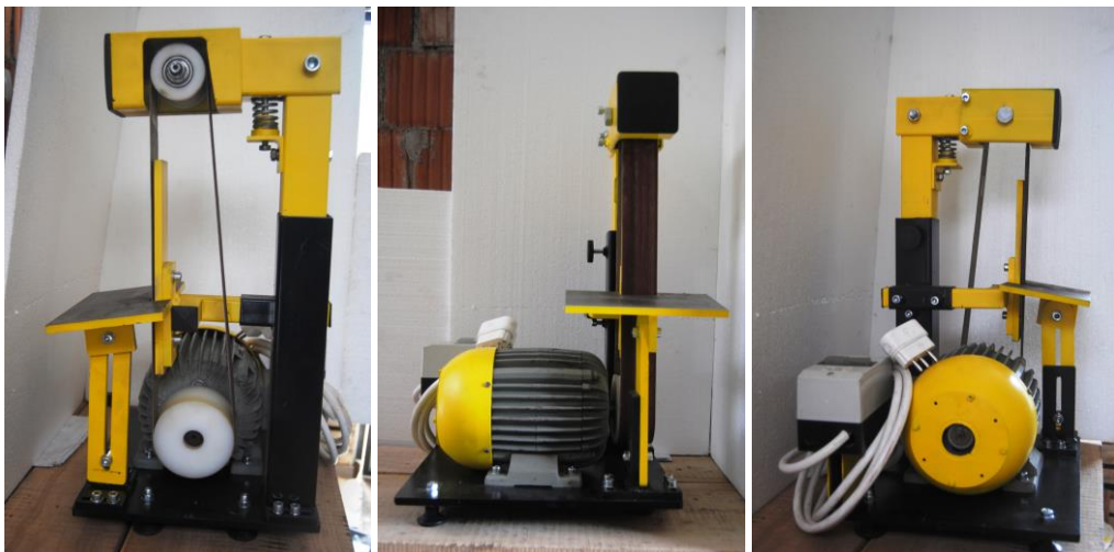
Figure 3. The fabricated belt grinder from different angles
