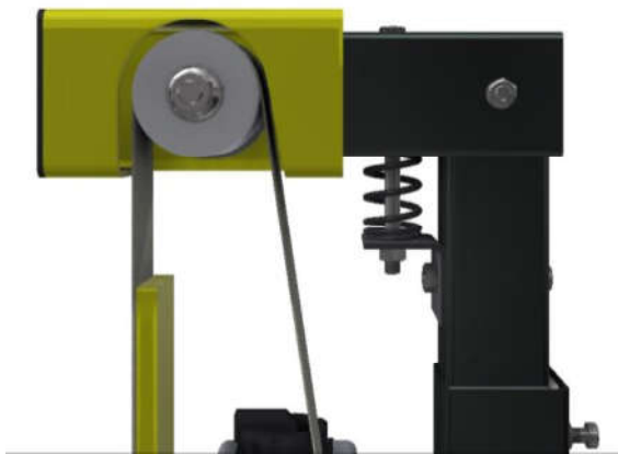
Fig.8. Tension mechanism of the solution 2
