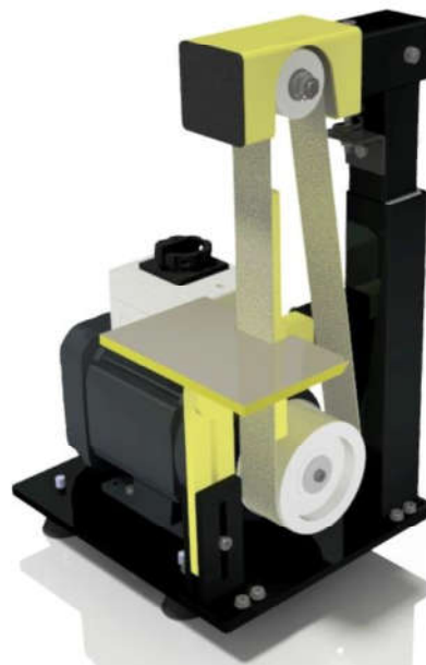
Fig.2. Belt grinder concept based steel plates and square steel pipes
