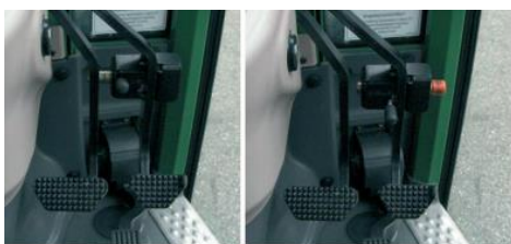
Figure 2 - Connected and disconnected command of tractor's brake
