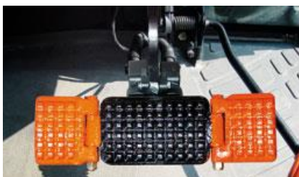
Figure 10 - New Holland's ABS SuperSteer brake-assisted steering will be operated by extensions to the single brake pedal [14]
