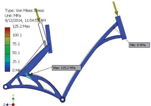
Fig.10. Von Mises stress of the second frame
