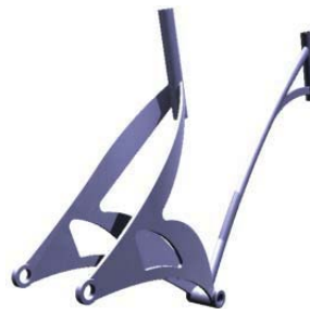
Fig.3. First bicycle frame CAD model
