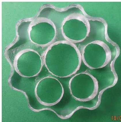
Figure 9 Cycloid disc produced on the milling machine 2Roland MDX-40A
