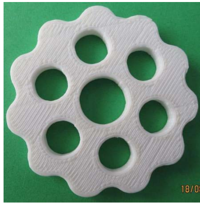
Figure 7 Cycloid disc printed on a 3D printer MakerBot Replicator 2
