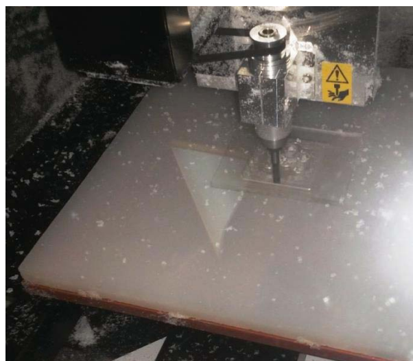
Figure 8 The method of production the model cycloid disc using milling machine Roland MDX-40A
