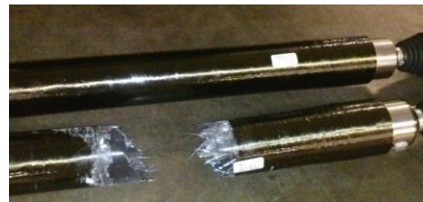
Figure 1- Fracture of one-piece composite drive shaft
