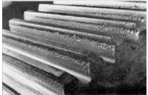
Fig. 1. Pitting of gear teeth 7
