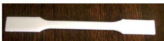
Figure 2. Specimens for testing of mechanical properties
