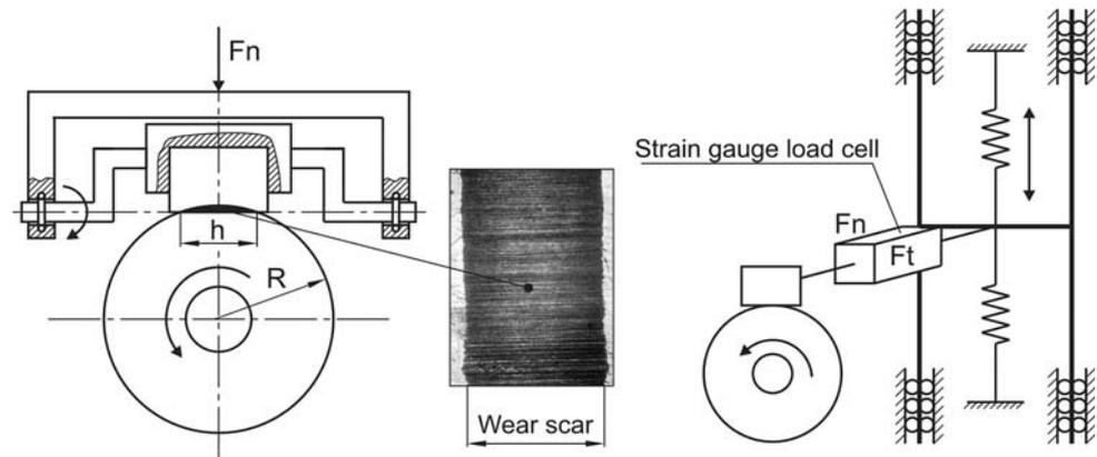
and sliding speeds was done in order to cover, by their combination at the given contact geometry, the regimes of the boundary and mixed lubrication. Those are the regimes in which mainly operate the bearings that are made of the ZA alloys. The duration of tests was 30 min (the sliding distance was 468 m). Tests were conducted with five repetitions.
