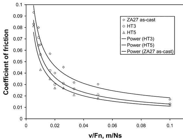
**Fig. 6** Friction coefficient of tested alloys versus speed-to-load ratio
