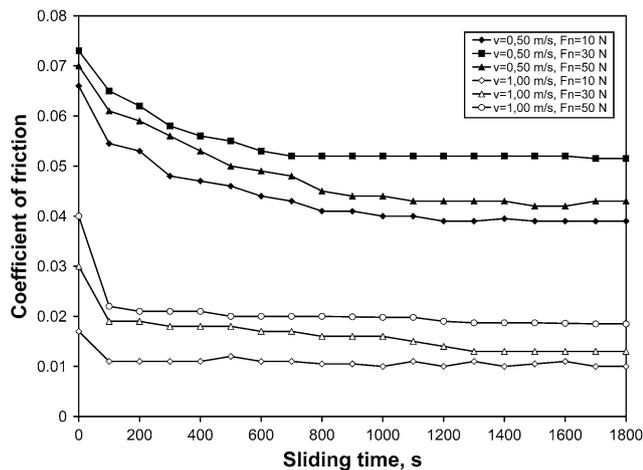
**Fig. 4** Friction coefficient variation of ZA27 HT5 alloy during sliding time at different specific loads and sliding speeds
