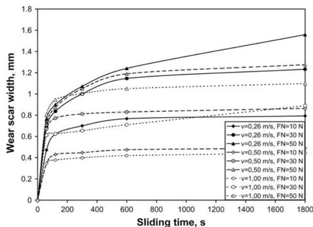
**Fig. 3** Wear curves of ZA27 HT5 alloy at different specific loads and sliding speeds
