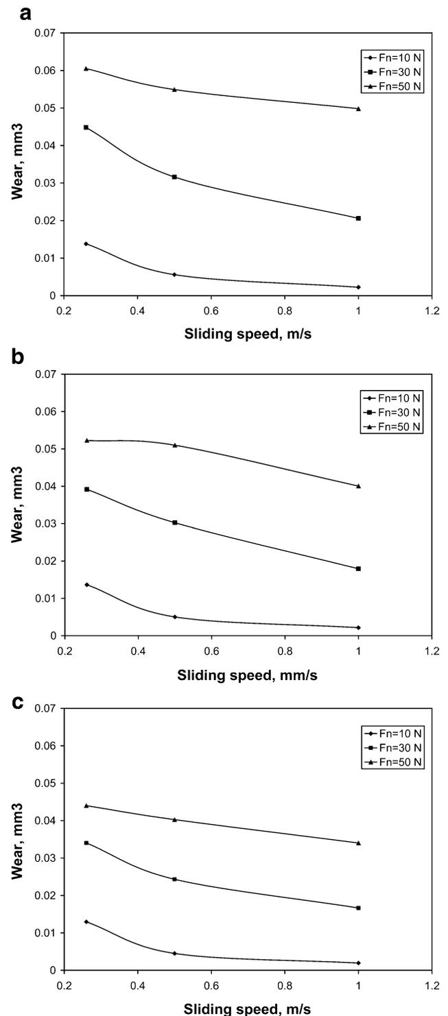
**Fig. 7** Wear loss of tested alloys versus sliding speed for different applied loads: **a** ZA27 as-cast, **b** ZA27 HT3, **c** ZA27 HT5
