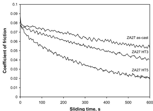
**Fig. 8** Friction coefficient of tested alloys versus sliding time for 30 N of applied load and 0.5 m/s of sliding speed
