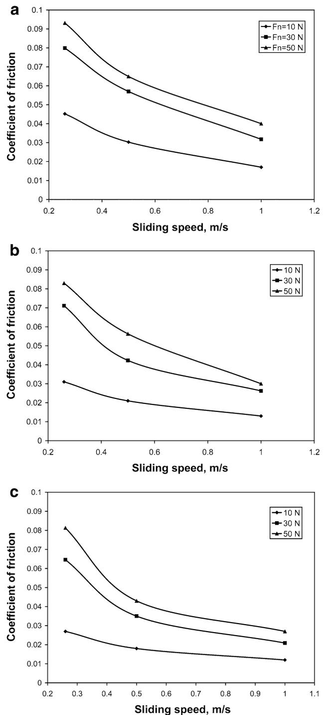
**Fig. 5** Friction coefficient versus sliding speed for different applied loads: **a** ZA27 as-cast alloy, **b** ZA27 HT3 alloy, **c** ZA27 HT5 alloy
