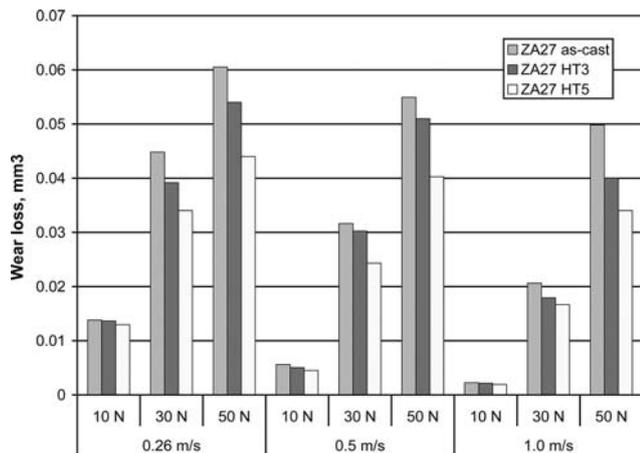
**Fig. 10** Wear volume loss of tested alloys comparison
