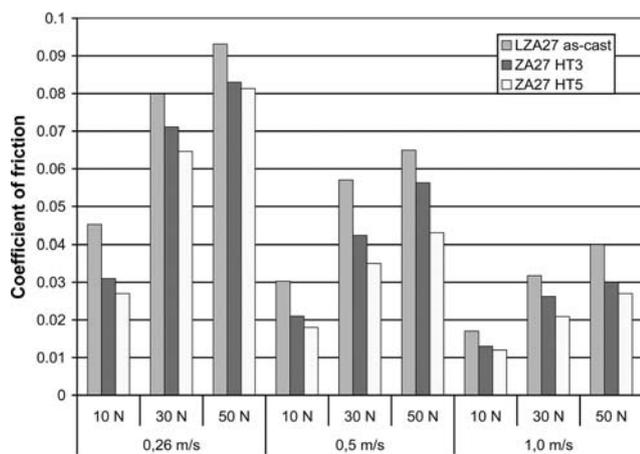
**Fig. 9** Friction coefficient of tested alloys comparison
