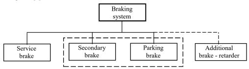
*Figure 1:* The structure of the braking system of a motor vehicle
