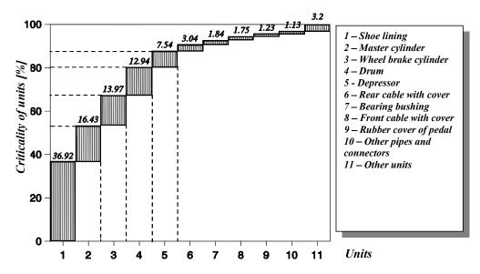
Figure 2: Pareto analysis of the absolute criticality degree of whole brake system
