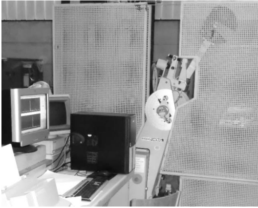
Fig. 5. Computerized Charpy pendulum used for testing
