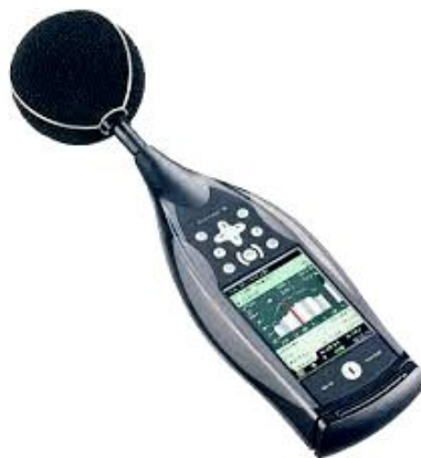
Figure 1. Sound Level Meter – Brüel & Kjær Type 2270
