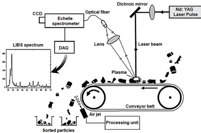
Figure 4. Components of a LIBS sorting system [16]
