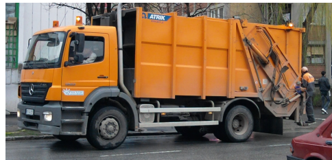
Figure 4. Solid waste collection vehicle with rear loadings and compactor in Kragujevac
