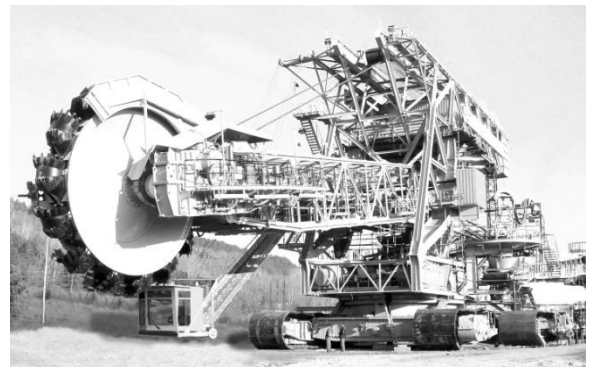
Fig. 1. Bucket-wheel excavator by FAM at Kolubara, Serbia
