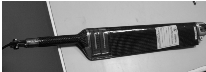
Figure 6: Strain gauges for continual monitoring of working characteristic with telemetry [3]
