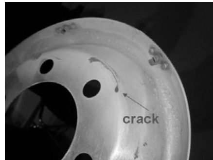
Figure 1: Example of penetrant nondestructive testing method [3]
