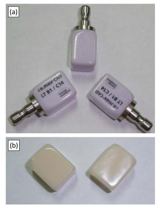
Figure 1. Lithium disilicate blocks (IPS e.max CAD): (a) partially crystallized blocks and (b) final state of crystallized blocks
