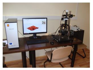
Figure 3. NT-MDT Atomic Force Microscopy (AFM), at the Tribology Center on the Faculty of Engineering in Kragujevac
