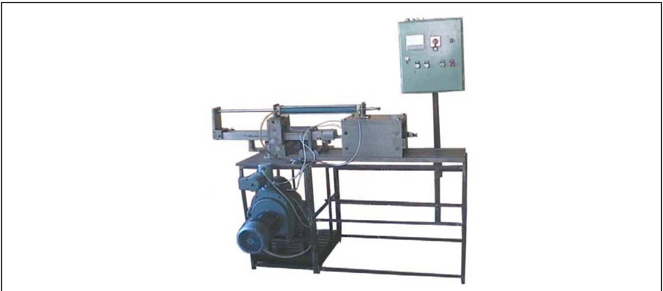
Figure 9. Device for testing the slide ways
