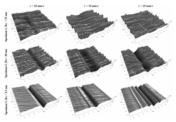
Figure 4. Morphology of the worn zones generated on TiN coatings of different roughness by reciprocating sliding with different sliding speeds
