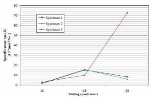
Figure 6. Specific wear rate of TiN coatings with different roughness in function of sliding speed
