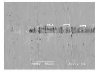
Figure 3. SEM micrograph of worn channel generated on Specimen 2, F=100mN, v=10mm/s
