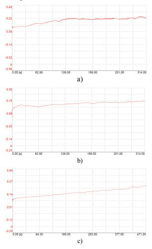
Figure 1. Evolution of the friction coefficient for different specimens, v=15mm/s, F=100mN
