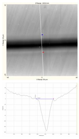
According to the SEM and AFM analyses there was no sign of wedge formation during wear. A wedge, which should be generated at the end of the wear track, forms when brittle coating is unable to absorb the load by its plastic deformation.
