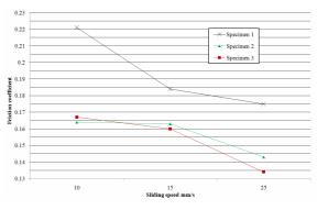
Figure 2. Friction coefficient of TiN coatings with different roughness in function of sliding speed
