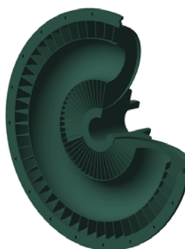
Sl. 7. 3D model pumpnog i turbinskog dela hidrodinamičke spojnice Fig. 7. 3D model of the impeler and the turbine of the hydrodynamic coupling
